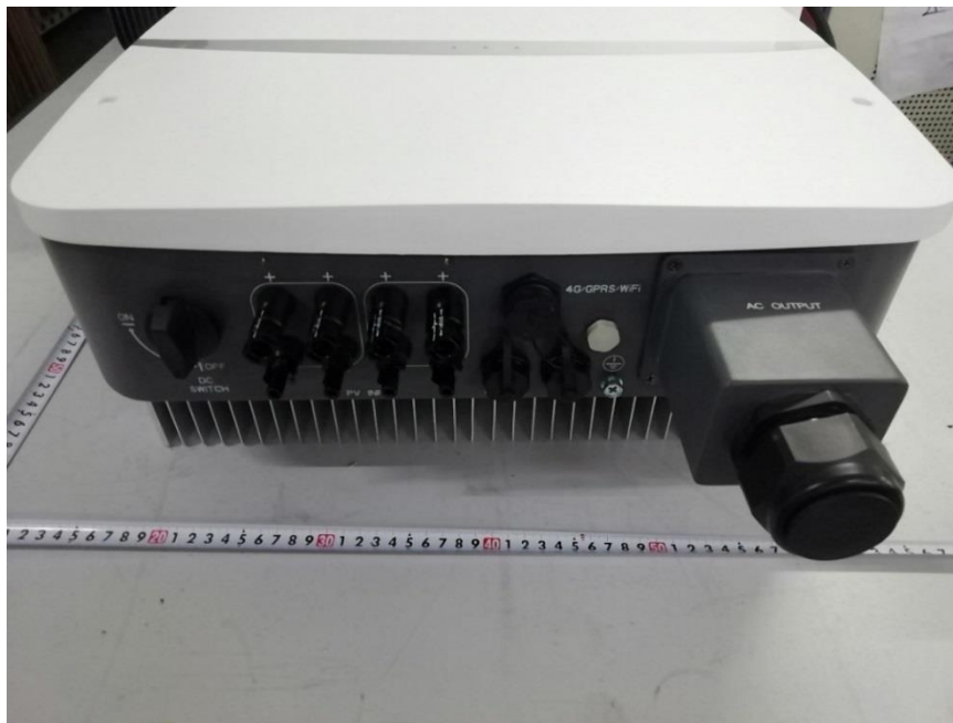
Figura 12. Vista em painel de conectores de R5-17K-T2 e R5-20K-T2 Figure 12. Connector panel view of R5-17K-T2 and R5-20K-T2
