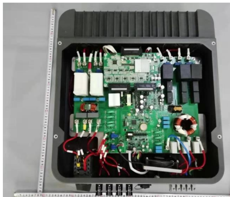
Figura 16. Vista interna para R5-17K-T2, R5-20K-T2 Figure 16. Internal view for R5-17K-T2, R5-20K-T2
