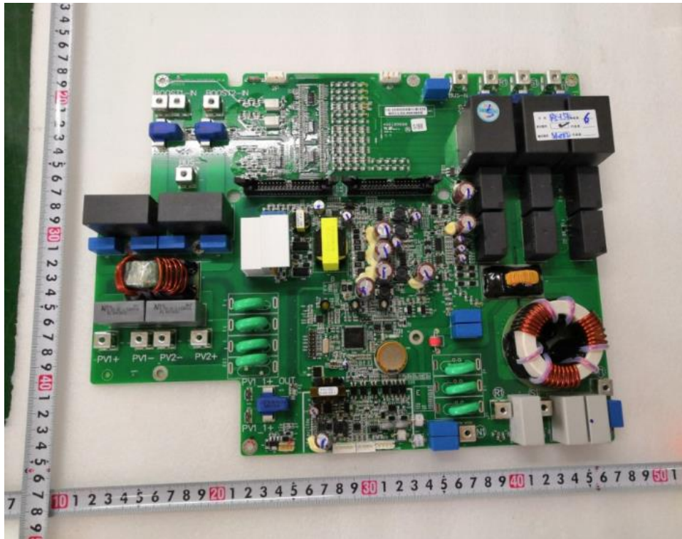
Figura 7. Vista frontal da placa de entrada / saída para R5-13K-T2, R5-15K-T2 Figure 7. Front view of the input/output board for R5-13K-T2, R5-15K-T2
