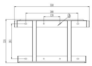
Figure 4.5 Dimensions of rear panel Suntrio Plus 40K/50K/60K
