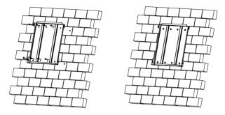
Figure 4.9 Mount the rear panel
