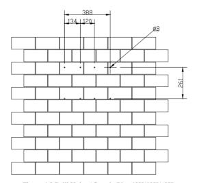
Figure 4.8 Drill Holes (Suntrio Plus 40K/50K/60K)
