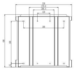
Figure 4.4 Dimensions of rear panel Suntrio Plus 25K/30K/33K
