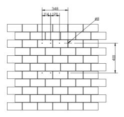
Figure 4.6 Drill holes (Suntrio Plus 12K/15K/17K/20K)
