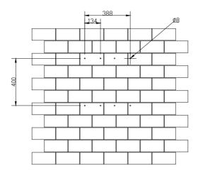
Figure 4.7 Drill Holes (Suntrio Plus 25K/30K/33K)
