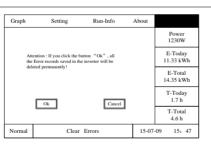
2. Press ▼and then press ENT to enter into "Clear Fault Records", click OK or return back.
