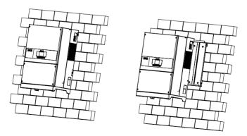
Figure 4.10 Mount the inverter
