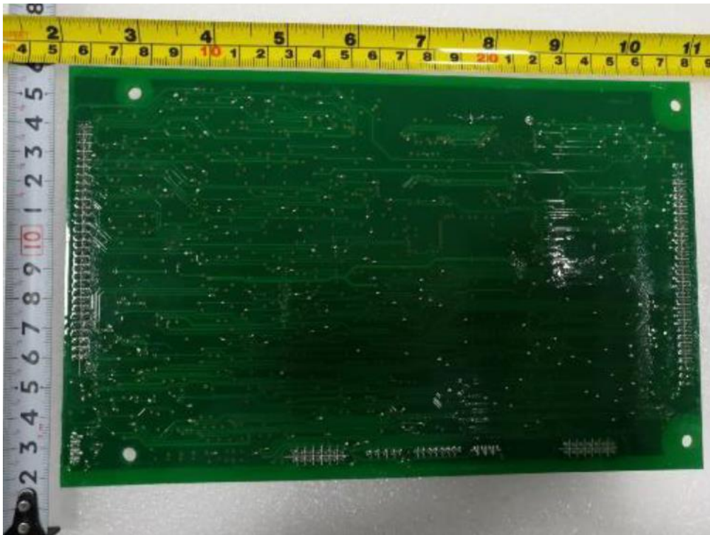
Figura 11 costas da painel de controle Figure 11 control board back
